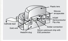
Fig 8: LED Operation (Source: E Source Lighting Atlas)
