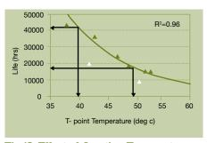
Fig 12: Effect of Junction Temperature on Life of LED Lamp (Source: Lighting Research Institute)
