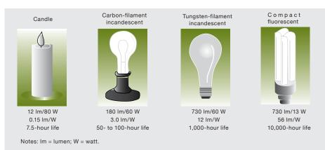
Fig 1: Evolution of Lighting Technologies (Source: E Source Lighting Atlas)
