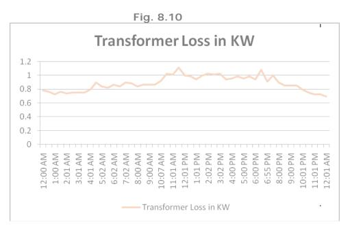
The load factor of Transformer varies from 10% to 28.1% The Power factor varies from 0.78 to 0.96 Lag
