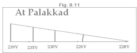
The voltage Drop is around 4.6%. This is within limit.
