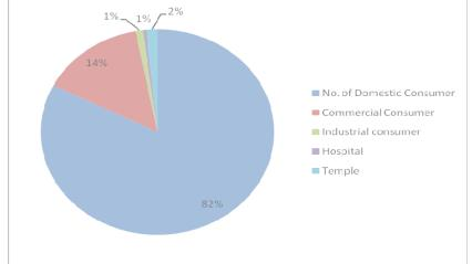
6.5.1 The consumer mix of this transformer may not have any impact on the distribution. There is only two small industrial loads and the significant loads are residential and partially commercial loads .The mix is in line with the total consumer mix of the entire Kerala State but the agriculture load is not there.
