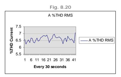
As per IEEE-519 – 1996 The THD for voltage at the connection point shall not exceed 5% with no individual Harmonics higher than 3%.
